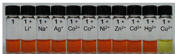
Figure 2. Pictures of 1 (0.025 mM) upon addition of various metal ions (5.0 equiv) in acetonitrile.
